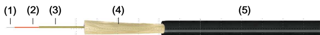
Figure 4 a) Main design features of the sensor cable (1) Quartz glass fibre, (2) Cladding, (3) Loose tube, (4) Aramid fibres, (5) Outer sheath
